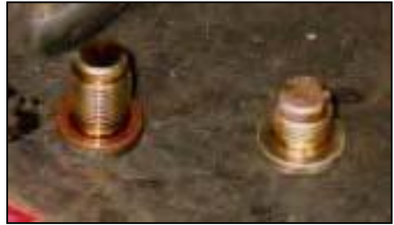
There are two types of sump plug depending on the age of your barchetta. Older cars will have the type shown on the right, whereas the one shown on the left is fitted to more recent cars.
